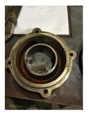
73. End Bell Air Seal Fits Drive End Air Seal
