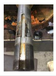
56. List the Parts needed for the Repair Below New shaft, and new bearings.
