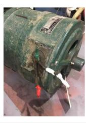
4. Describe the Overall Condition of the Equipment as Received Received Stator and d.e housing only.
