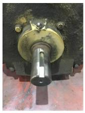
7. Assembled Shaft Runout 0.003 Inches
