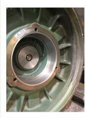
85. Bearing Cap Condition Post Repair
