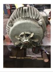
14. Broken or Missing Components
