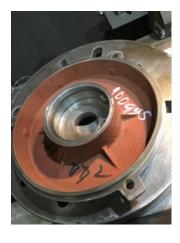
88. Bearing Cap Condition Post Repair
