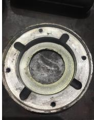
56. End Bell Air Seal Fits Opposite Drive End Air Seal Drive End Air Seal
