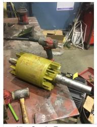
37. Growler Test (Pass) Pass38. Number of Rotor Bars
