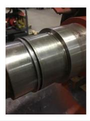
Drive End Bearing Shaft Fit Condition (F) Fail
