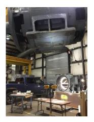
Describe the Overall Condition of the Equipment as Received Windings need to be steamed and baked Bore and Bush on both endbells
