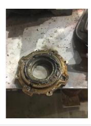
4. Describe the Overall Condition of the Equipment as Received Fan broken, four ea. fan cover mount bolts broken off. Coupling has wear on aft end.
