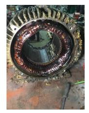
4. Describe the Overall Condition of the Equipment as Received *Filthy: Covered with sticky grease like substance.*
