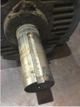
7. Assembled Shaft Runout
