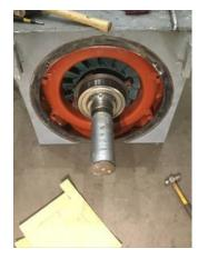
88. Final Insulation Resistance Test
