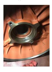
Drive End Bearing Cap Opposite Drive End Bearing Cap
