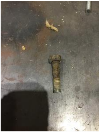
Mount bolts corroded and need replacing.
