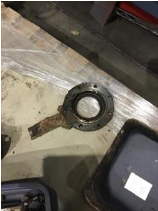
Mount bolts corroded and need replacing.
