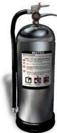
Water is one of the most commonly used extinguishing agents for type A fires. You can recognize an APW by its large silver container. They are filled about two-thirds of the way with ordinary water, then pressurized with air. In some cases, detergents are added to the water to produce a foam. They stand about two to three feet tall and weigh approximately 25 pounds when full.
