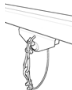
Diagram 11C. Safety cable installed on Gorbels® trolley that will attach to hoist (by others).
