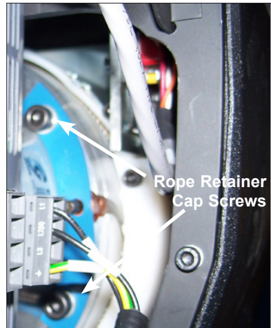
Diagram S. Remove the two M8 socket head cap screws and slide retainer off of rope end towards you.
