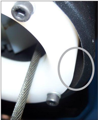
Diagram M. Insert screwdriver between the white wear ring and the actuator casting where the rope exits the actuator.
