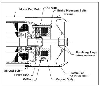
Figure 6: Motor Brake
