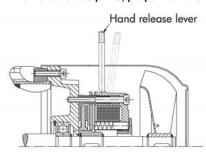
ments must be made in the field. Hand-lever adjustments must always be made prior to assembling the brake to the motor. All brake air gap adjustments must be made with the brake assembled to the motor and the power off (brake engaged).
