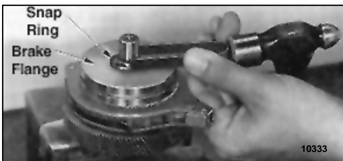
Figure 5-6. Remove Snap Ring From Load Brake Shaft
