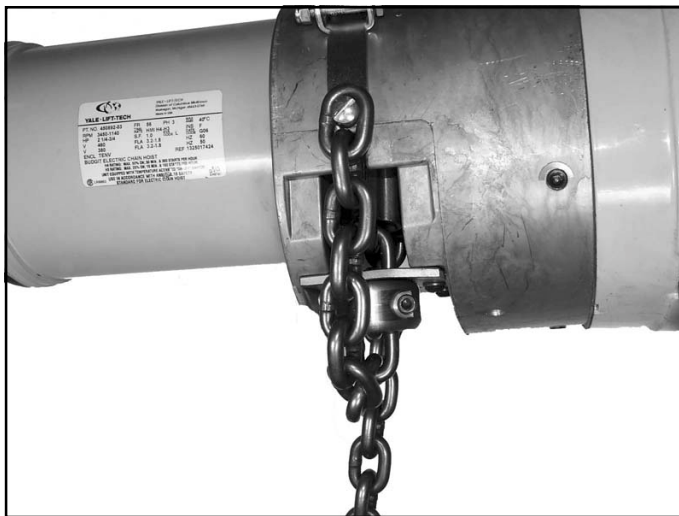
Figure 3-2. Actuator Contacting Stop Tail Chain End of Load Chain
