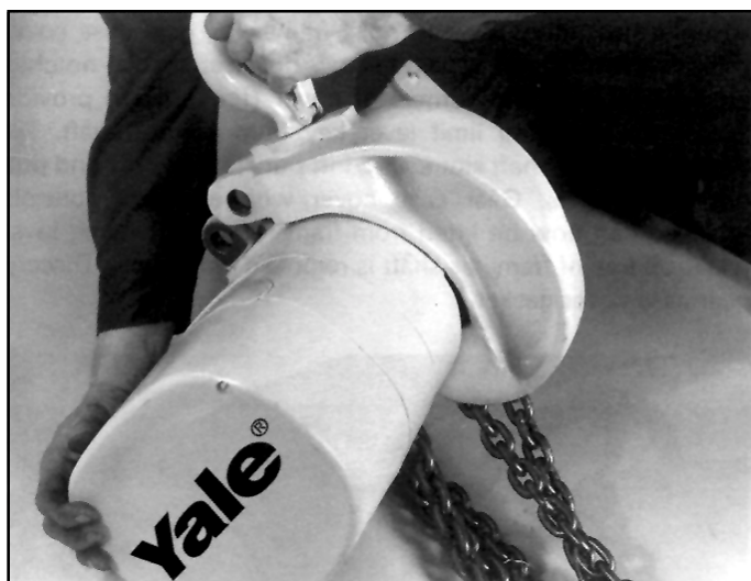
Figure 7-3. Removing 3 Ton Hanger Bracket from Hoist Frame
