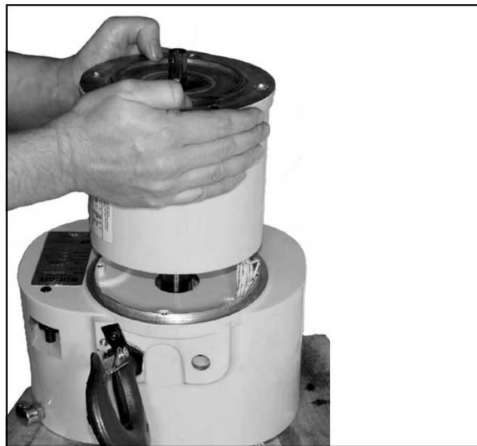
Figure 7-9. Removing Motor Assembly
