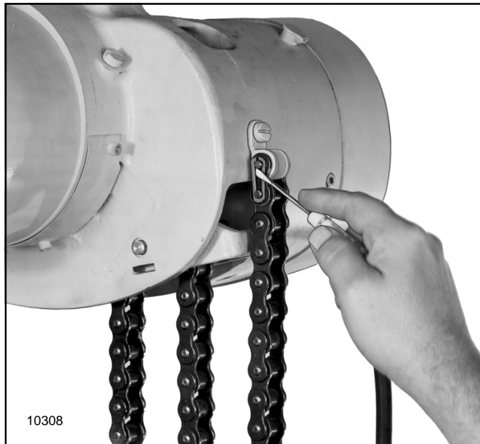
Figure 7-1. Removing Spring Clip from Connecting Link at Tail End of Load Chain (Roller Chain Models)
