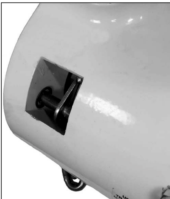
Figure 7-13. Removing Chain Guide Support Pins
