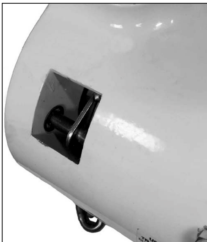
Figure 7-13. Removing Chain Guide Support Pins
