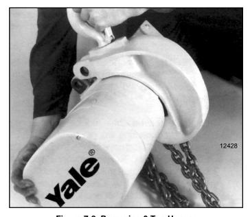
Figure 7-2. Removing 3 Ton Hanger Bracket from Hoist Frame
