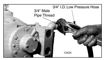
Figure 2-1. Connecting Air Hose to Hoist
