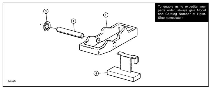
Figure 8-6. LIMIT STOP AND PARTS
