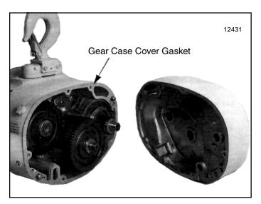
Figure 7-5. Gearcase Cover Removed From Hoist Frame
