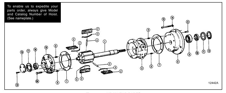
Figure 8-8. AIR MOTOR PARTS
