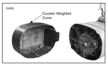
Figure 7-3. View of Hoist with Counterweighted Compartment Cover Removed
