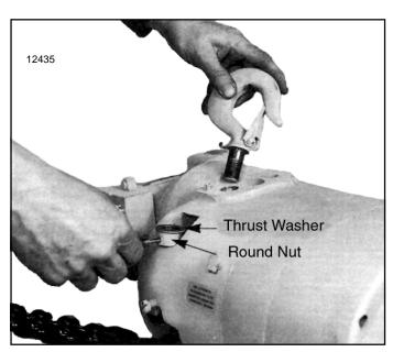
Figure 7-17. Removing Suspension Lug (Single Reeved Model)
