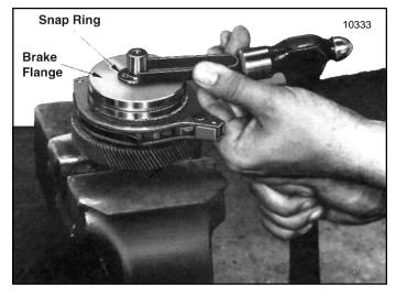
Figure 7-18. Removing Snap Ring from Load Brake Shaft
