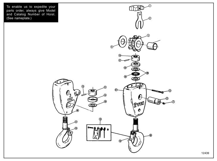
Figure 8-5. 2 & 3 TON LOWER BLOCK ASSEMBLIES
