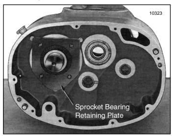
Figure 7-10. View of Sprocket Bearing Retaining Plate
