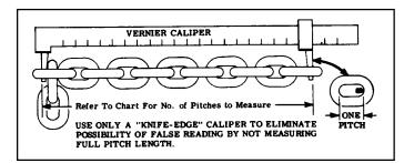
Figure 5-2. Check Coil Chain Using Vernier Caliper
