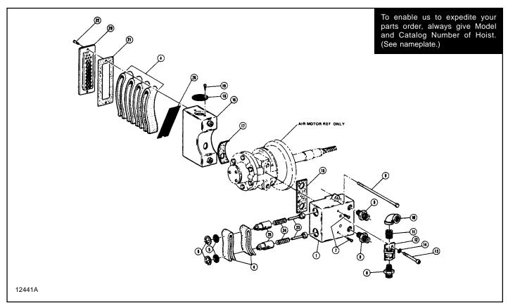
Figure 8-7. SUPPLY HEAD AND MUFFLER PARTS
