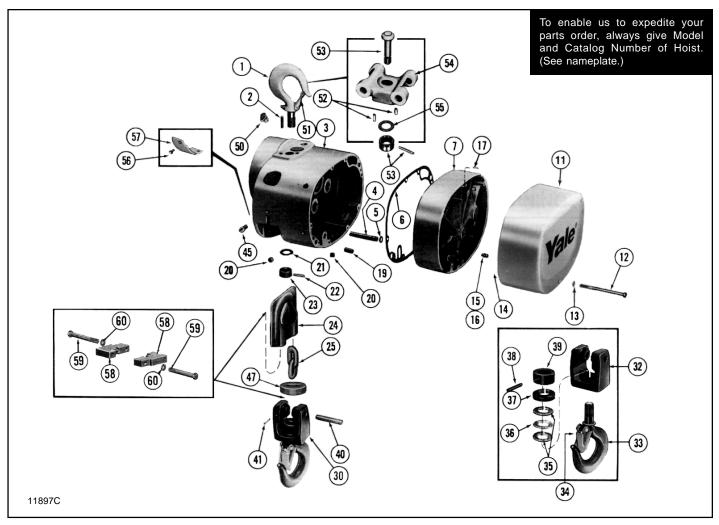
Figure 8-1. FRAME AND EXTERNAL PARTS
