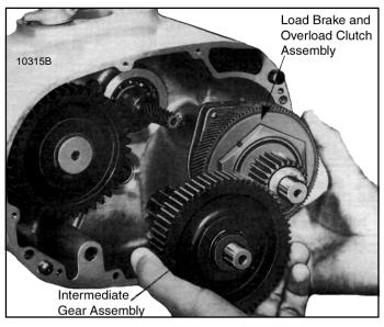
Figure 7-7. Removing Load Brake and Clutch and Intermediate Gear Subassemblies
