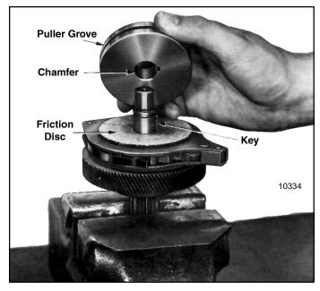
Figure 7-19. View Showing Load Brake Flange Removed
