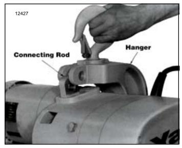
Figure 7-1. 3 Ton Hanger Bracket Connection Pin Removed
