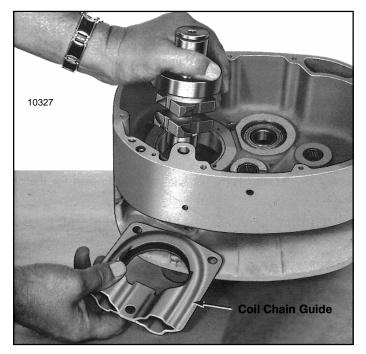
Figure 7-14. Chain Guide Being Removed From Frame as Sprocket Shaft is Lifted Out
