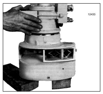
Figure 7-8. Removing Motor Assembly
