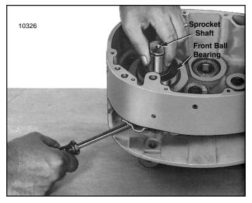
Figure 7-13. Removing Sprocket Shaft and Front Bearing
