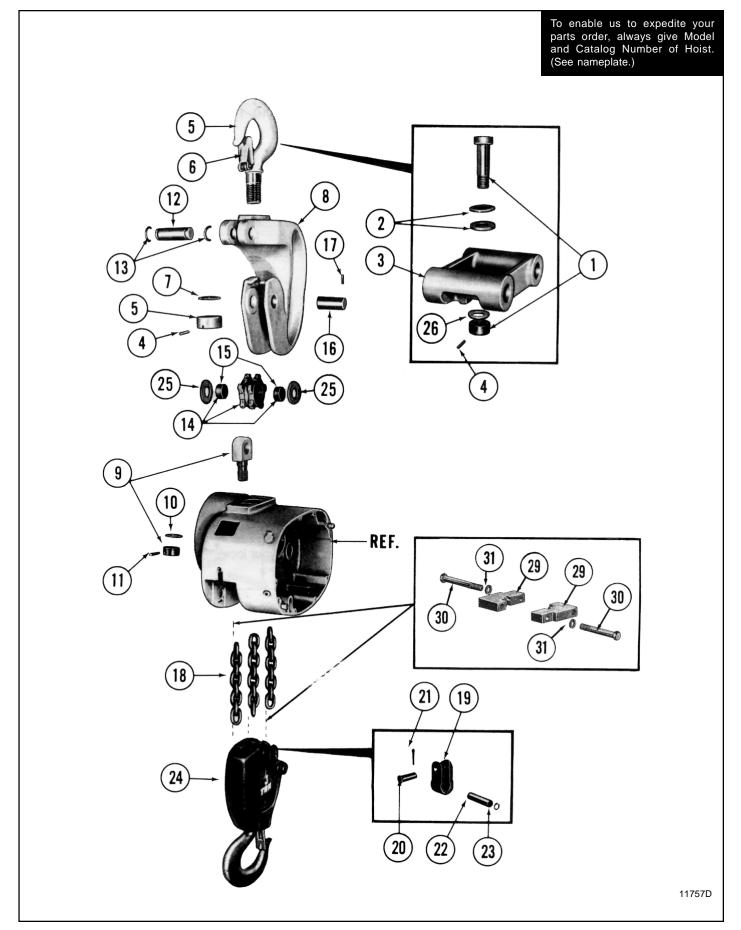
Figure 8-3. UPPER SUSPENSION, LOAD CHAIN AND LOWER BLOCK PARTS (3 ton Capacity Hoists)
