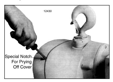
Figure 7-4. Prying Gearcase Cover From Hoist Frame
