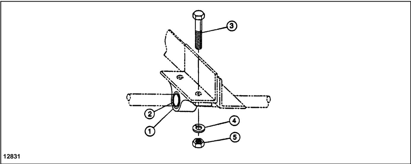
Figure 3. Cross Shaft Bearing Assembly. (Catalog Number 904625).
