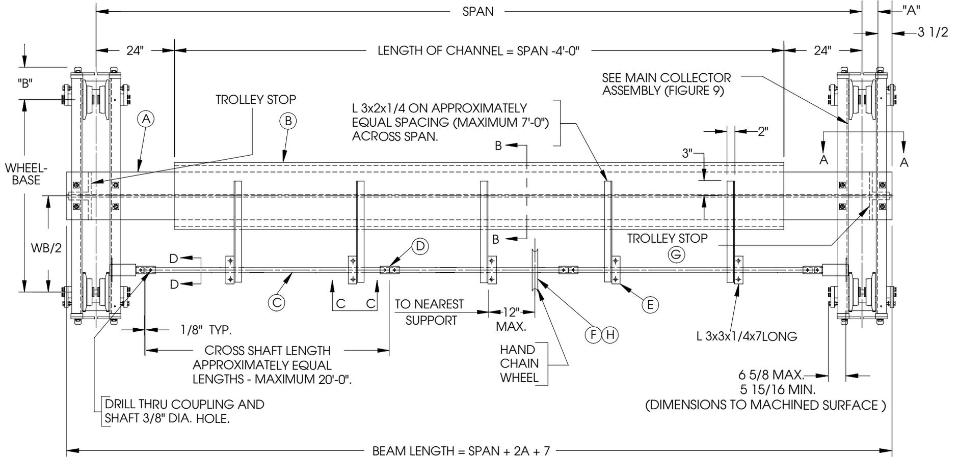
SEE FIGURE 10. FOR DIMENSIONS A AND B, SECTIONS A-A, B-B, C-C, D-D, AND ITEMS E AND G.
