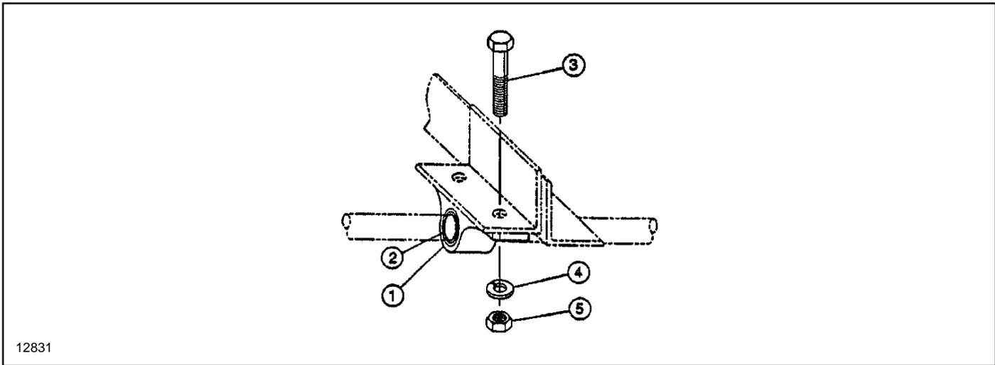
Figure 2. Cross Shaft Bearing Assembly. (Catalog Number 904625)
