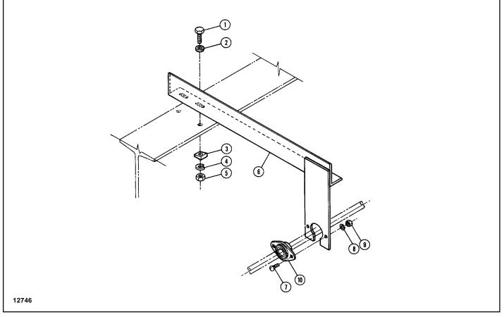
Figure 13. Cross Shaft Support. Catalog Number 904540.
