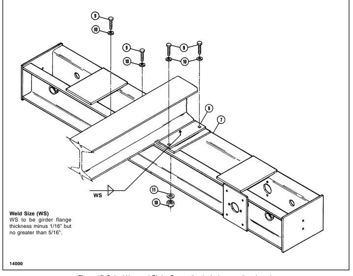
Figure 17. Bolted Uncoped Girder Connection (only 1 connection shown).
