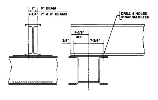
Figure 6. Bridge Beam End Connections.
