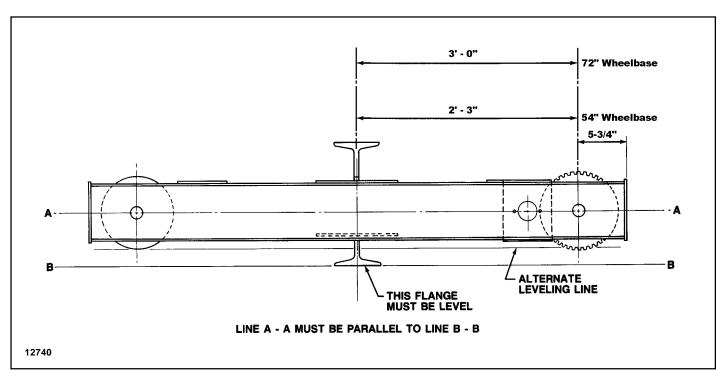
Figure 5. Method of Setting End Truck to Girder.
