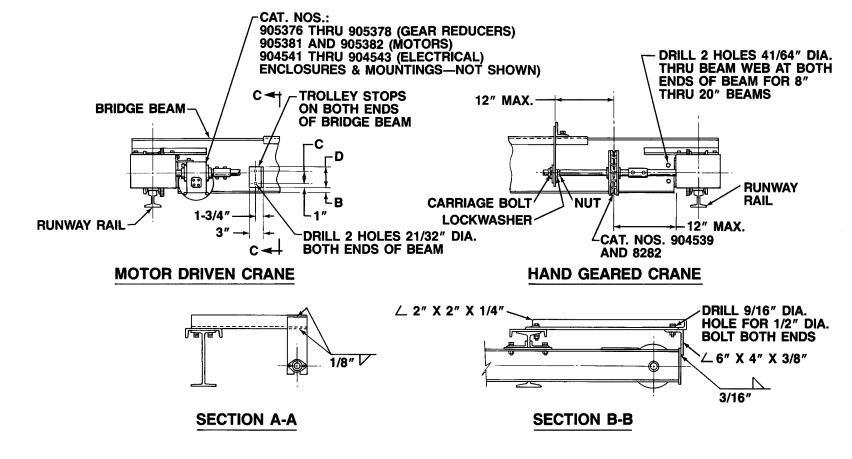
\*Trolley frame or bumpers should contact trolley stops. If not, cut out standing leg (OSL) back to dimension shown.
