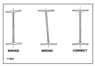
Figure 2. Correct Beam Selection.
