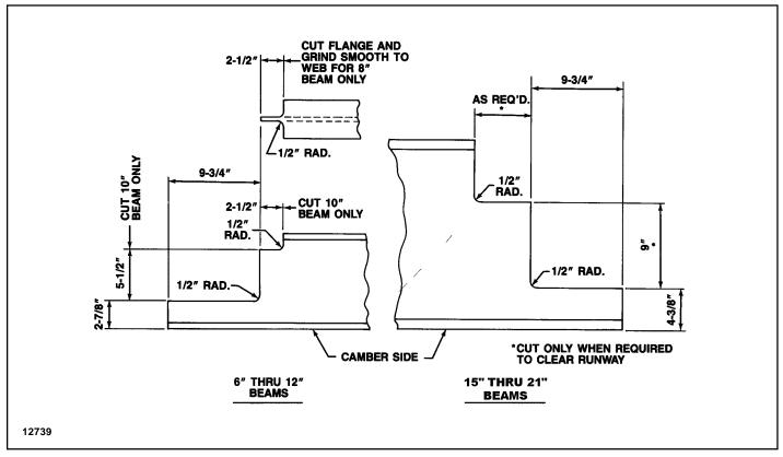
Figure 4. Cutting Diagram.
