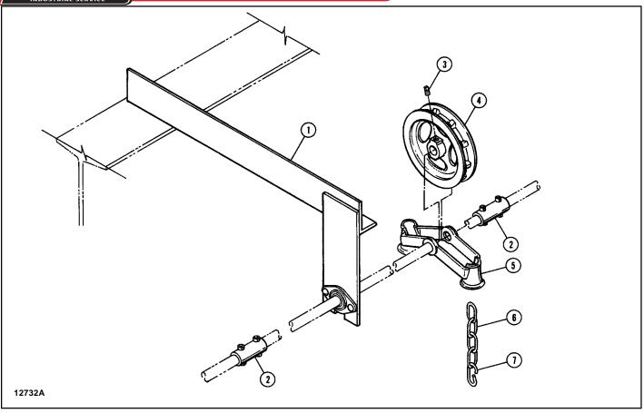
Figure 15. Hand Chain Drive. Catalog Numbers 904539 and 8282.
