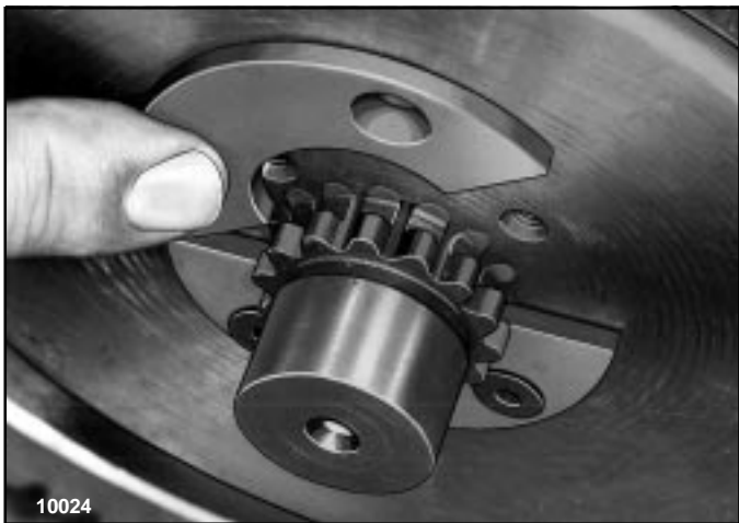
Figure 8-7. Removing Retainer Plates on Load Brake Shaft.
