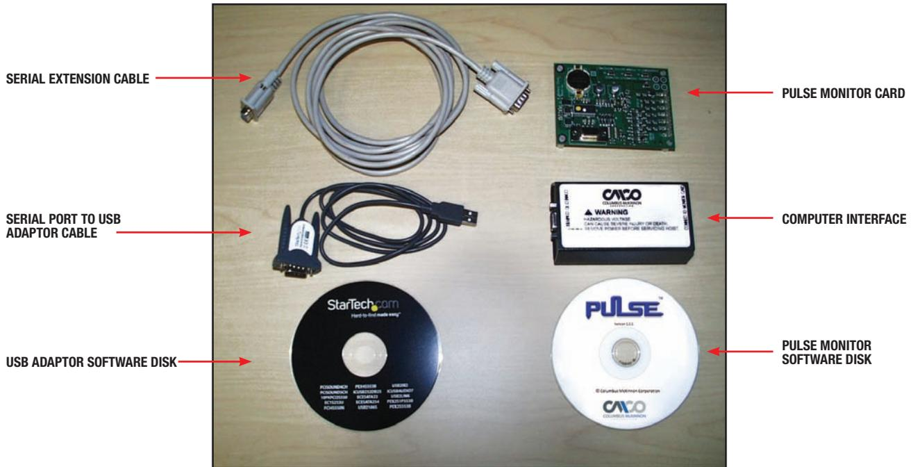
**Note:** Kit also includes a DB9 to DB25 pin adapter for 25-pin RS232 serial communication which will not be needed in most cases.
