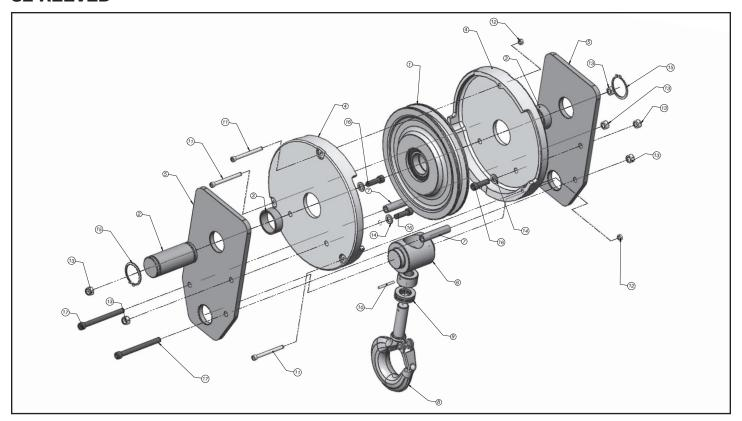
Figure 9-4b. Lower Block Assembly (S2 Reeved)
