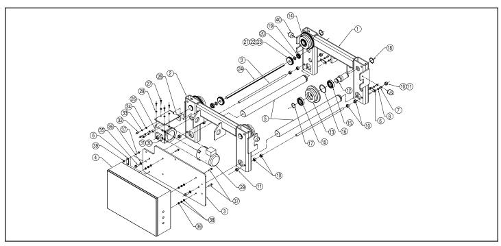
Figure 9-3. Motor Driven Trolley Frame and Drive (S4 Reeved "C" Frame Shown).
