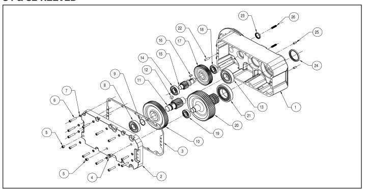
Figure 9-2. Hoist Gearing
