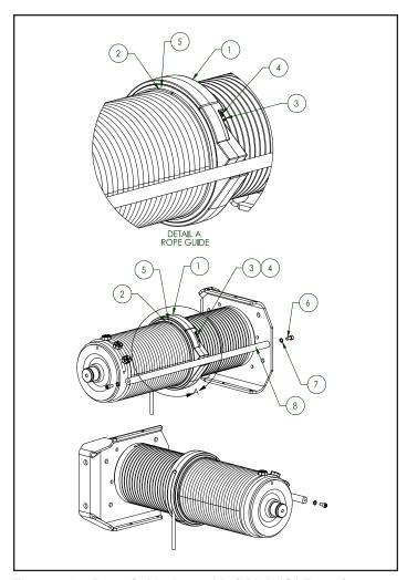
Figure 5-3a. Rope Guide Assembly ("B" & "C" Frame)
