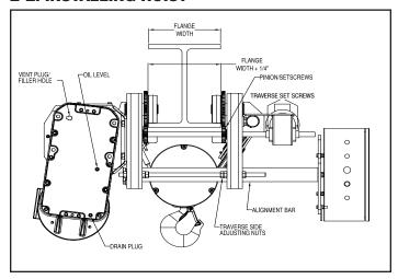
Figure 2-1. Trolley Wheel Spacing ("B" & "C" Frame Shown)
