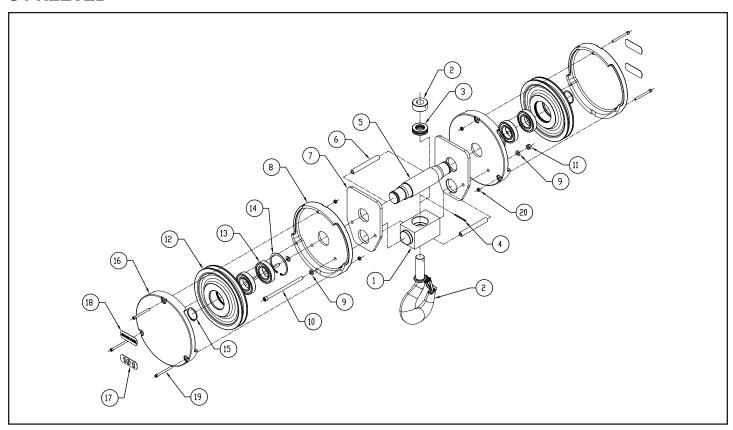
Figure 9-4a. Lower Block Assembly (S4 Reeved)
