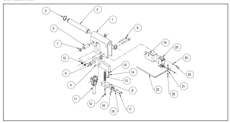
Figure 9-6c. Wire Rope Dead End Assembly with Limit Switch ("B" & "C" Frame) (S2 Reeved)
