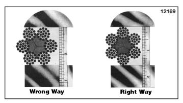
Figure 5-4. Correct Method of Measuring Rope
