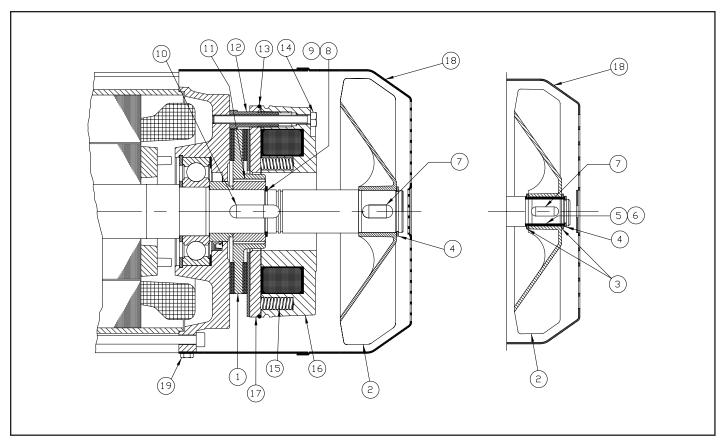
Figure 9-8b. Standard Hoist Motor Brake (ABM Motor)
