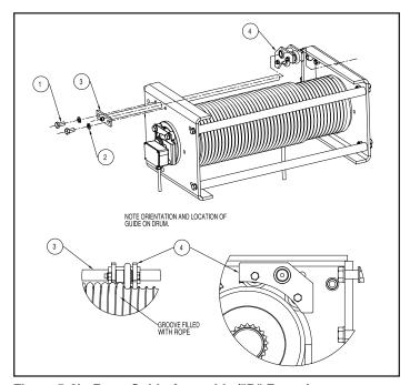
Figure 5-3b. Rope Guide Assembly ("D" Frame)
