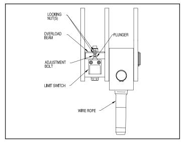
Figure 7-3b. Over-Capacity Limit Switch ("D" Frame)
