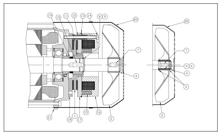
Figure 9-9a. Outdoor Service Hoist Motor Brake (ABM Motor)
