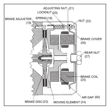
Figure 5-8b. MGM Motor Brake
