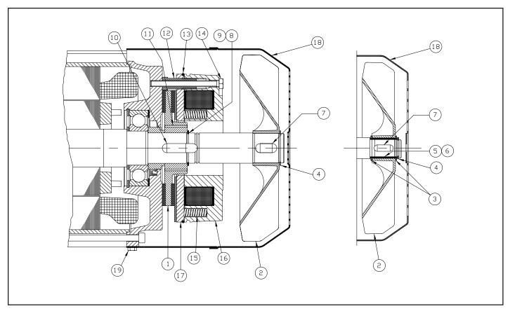
Figure 9-8a. Standard Hoist Motor Brake (ABM Motor)
