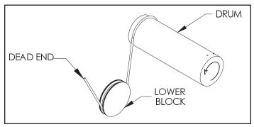
Figure 5-5a. Reeving Diagram - 2 Part Single Reeved. (Note: Arrow on Drum Indicates Direction of Drum when Lowering.)
