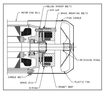
Figure 5-8a. ABM Motor Brake
