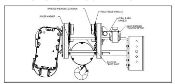
Figure 5-9. Traverse Drive Arrangement ("B" & "C" Frame Shown)
