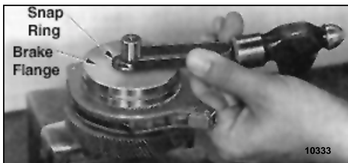
Figure 5-6. Remove Snap Ring From Load Brake Shaft
