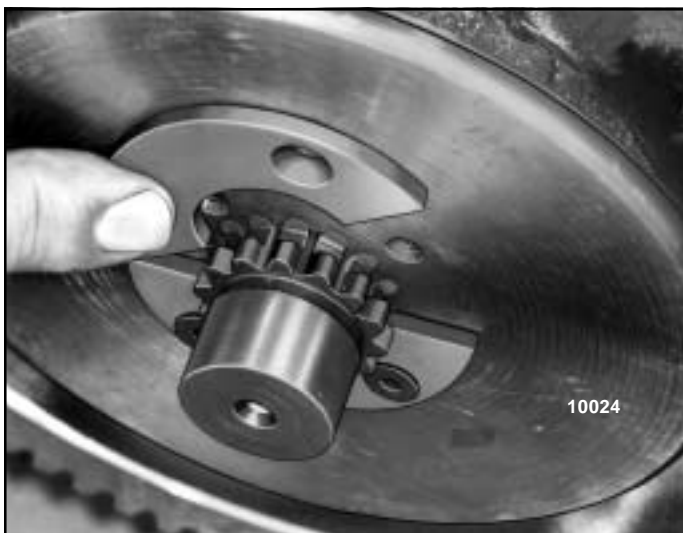
Figure 5-5. Installing Retainer Plates on Load Brake Shaft
