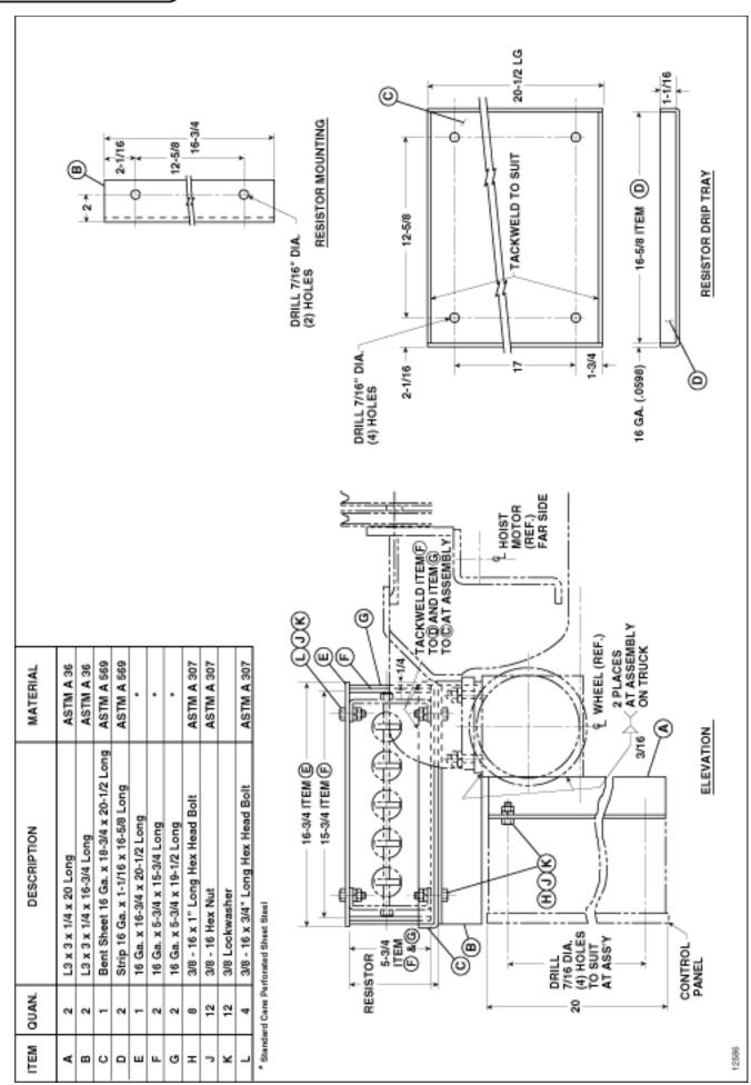
Figure C. Electrical Enclosure and Resistor Mounting Arrangement
