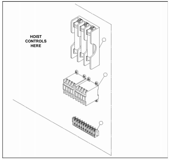
Figure 4. Traverse Controls for Single Speed Trolley.
