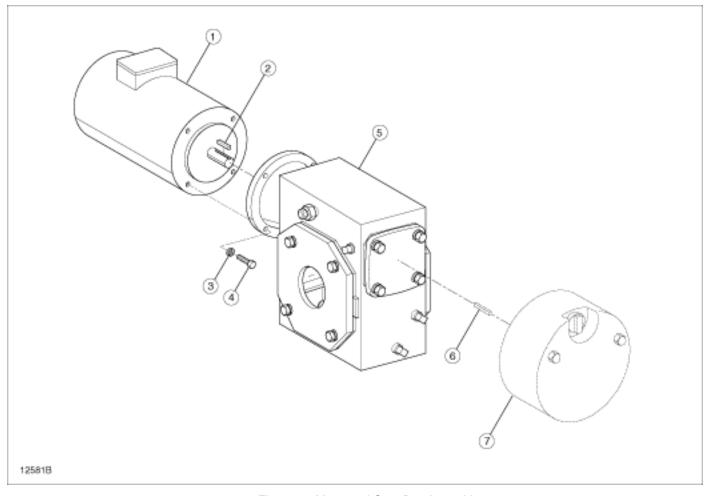
Figure 3. Motor and Gear Box Assembly.
