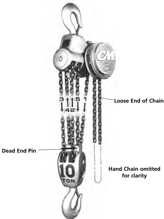
FIGURE 21. Reaving 10 Ton Hoists
