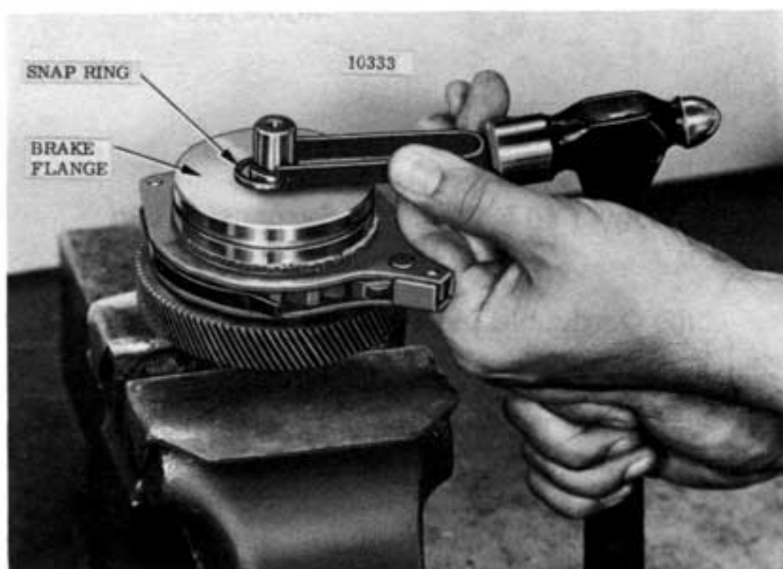
Figure 7-18. Removing Snap Ring from Load Brake Shaft.
