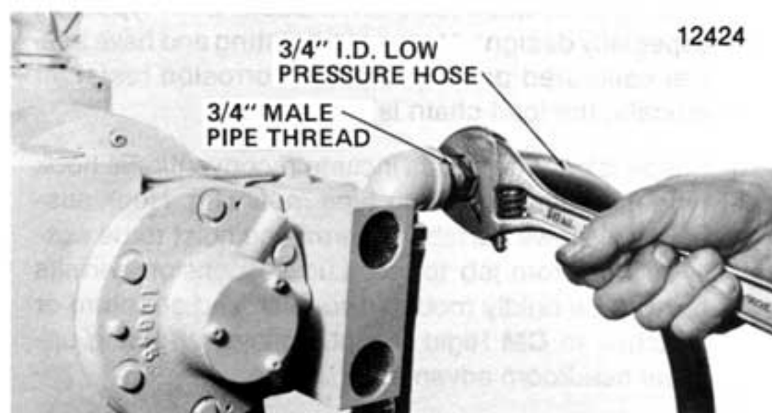
Figure 2-1. Connecting Air Hose to Hoist.
