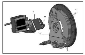
Reposition the support bracket assembly (3) on the brake, and retighten the two support bracket screws (35), (52 lb-in).
