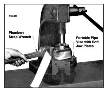
Figure 7-25. Winding Load Brake Gear Using a Strap Wrench to Set Up Load Brake Spring
