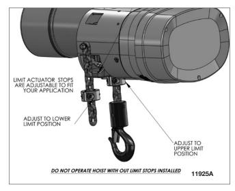
Figure 3-1. Limit Switch Illustration
