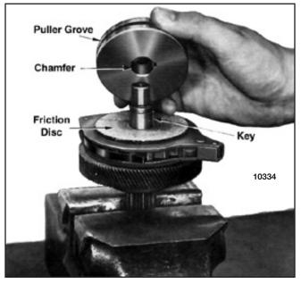
Figure 7-22. View Showing Load Brake Flange Removed
