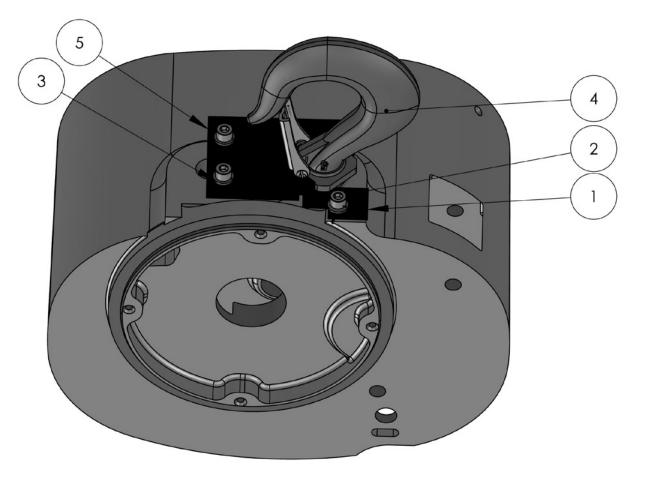
Figure 9-2A. UPPER SUSPENSION, 1/4 TO 1 TON HOOK
