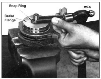
Figure 7-21. Removing Snap Ring from Load Brake Shaft
