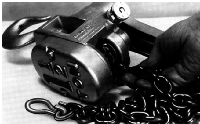
Figure 13. Chain Assembly - Hook End, 1 1/2 Ton
