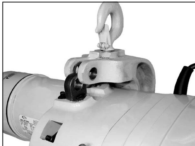
Figure 7-2. 3 Ton Hanger Bracket Connection Pin Removed
