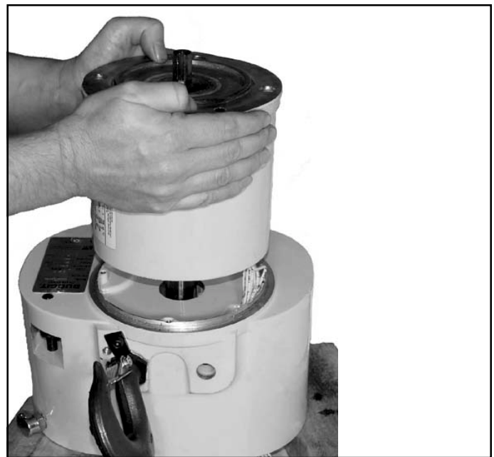
Figure 7-9. Removing Motor Assembly
