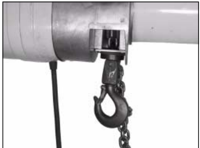
Figure 3-1. Lower Block Contacting Stops at Upper Limit of Travel
