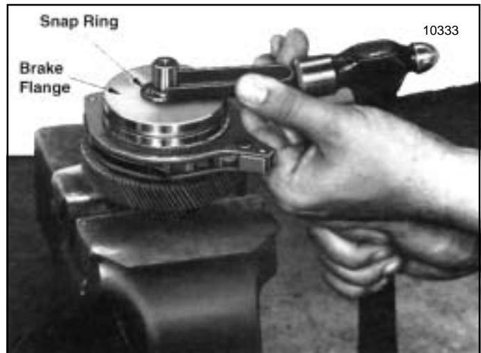
Figure 7-21. Removing Snap Ring from Load Brake Shaft
