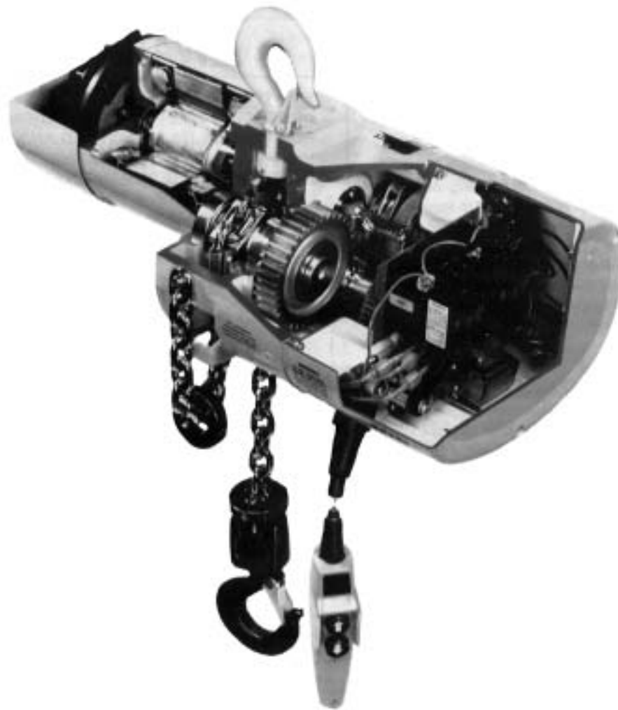
Figure 1-1. Cutaway View Of Typical Budgit Electric Hoist
