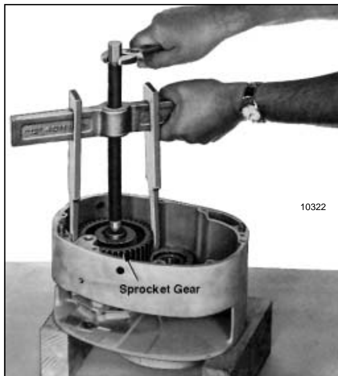
Figure 7-10. Pulling Sprocket Gear from Sprocket Shaft using Common Puller
