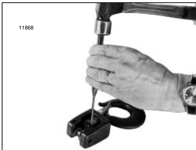
Figure 7-26. Removing Roll Pin Securing Hook Nut to Hook Shank
