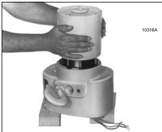
Figure 7-9. Removing Motor Assembly
