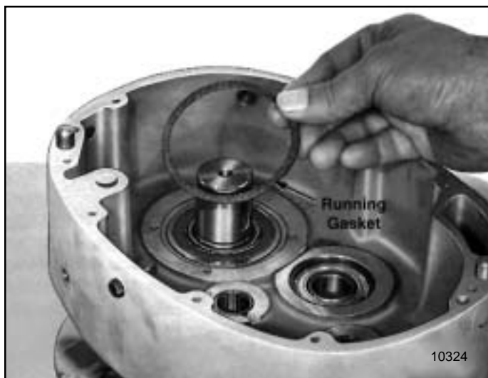
Figure 7-12. Removing Sprocket Bearing Ring Gasket. (On later model hoists ring gasket is replaced by a seal disk with oil seals)
