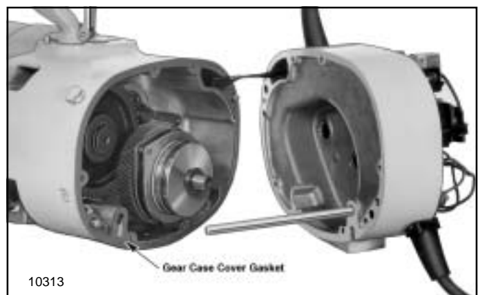
Figure 7-6. Gear Case Cover with Electrical Controls Removed from Frame
