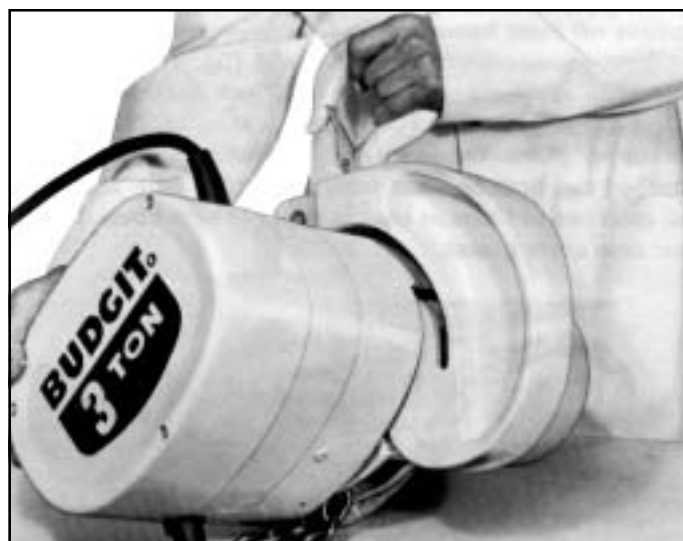
Figure 7-3. Removing 3 Ton Hanger Bracket from Hoist Frame
