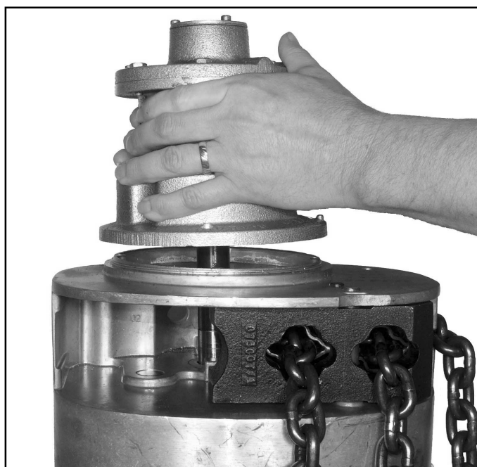
Figure 7-8. Removing Motor Assembly
