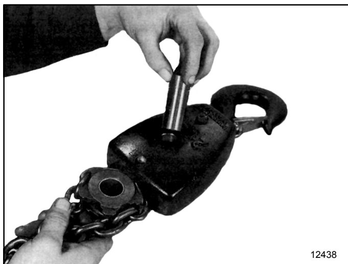
Figure 7-26. Removing Coil Chain and Sprocket on Double and Triple Reeved Lower Block Assembly
