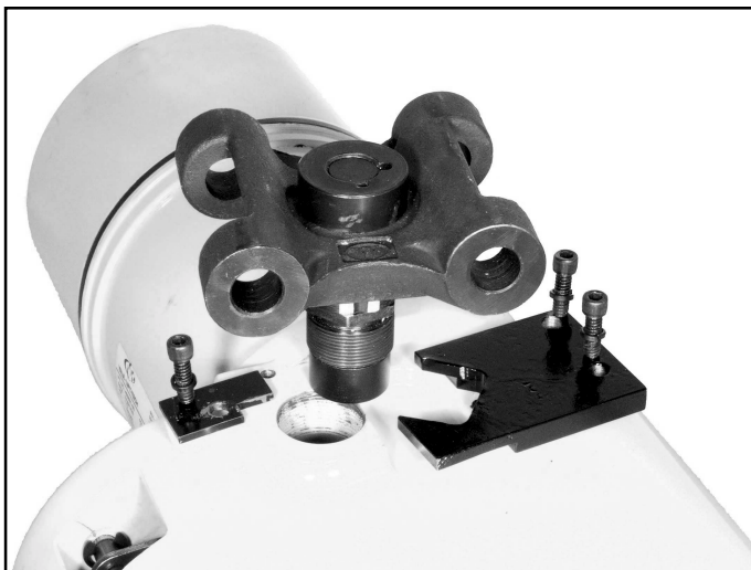
Figure 7-17. Removing Suspension Lug (1/4 through 1 Ton Models)
