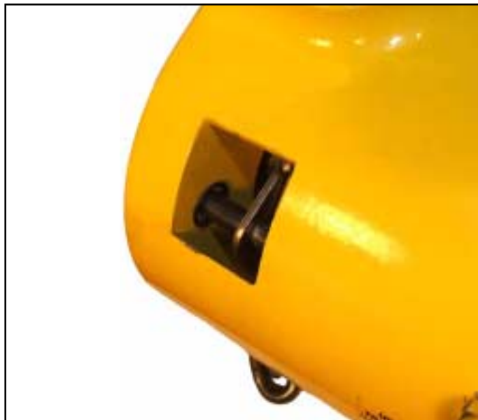
Figure 7-12. Removing Chain Guide Support Pins
