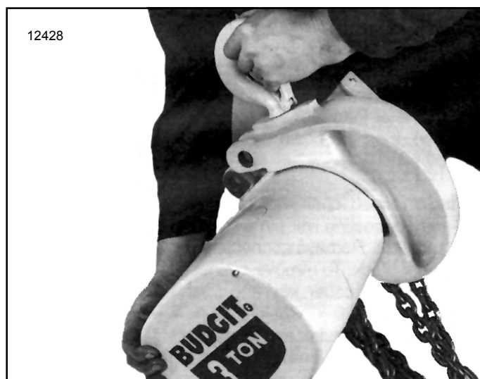
Figure 7-2. Removing 3 Ton Hanger Bracket from Hoist Frame
