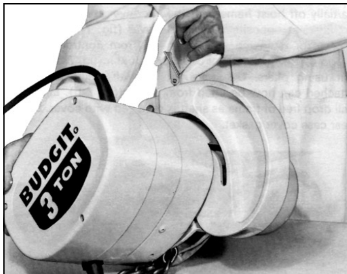
Figure 7-3. Removing 3 Ton Hanger Bracket from Hoist Frame
