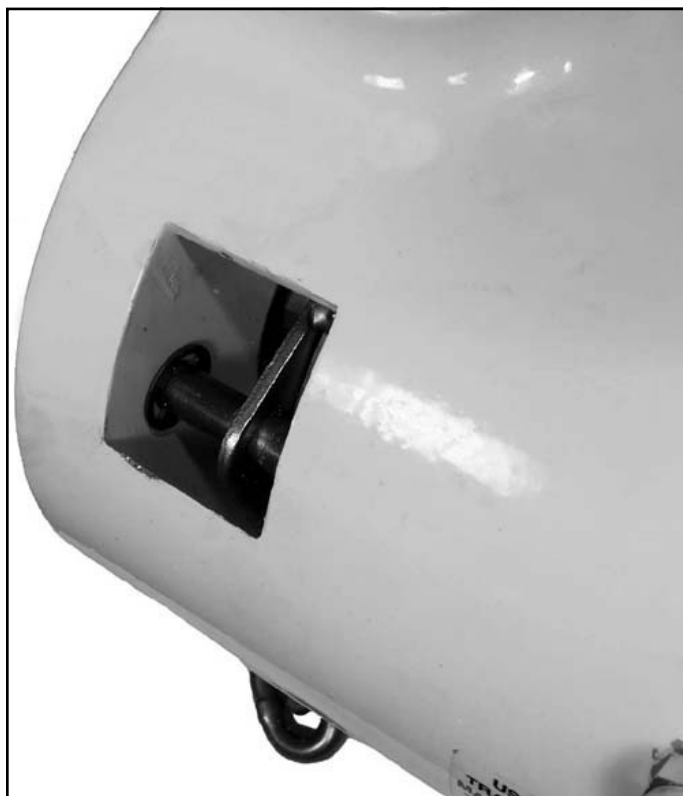
Figure 7-13. Removing Chain Guide Support Pins
