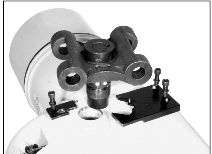
Figure 7-20. Removing Suspension Lug (1/4 through 1 Ton Models)
