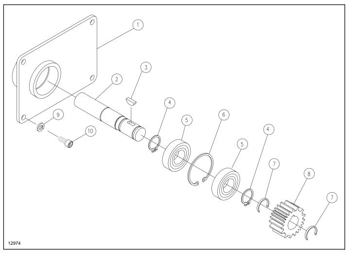
Figure 5. Hand Geared Drive Adapter
