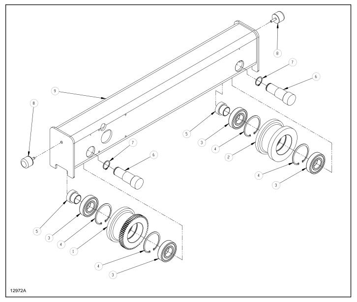
Figure 1. End Truck Assembly
