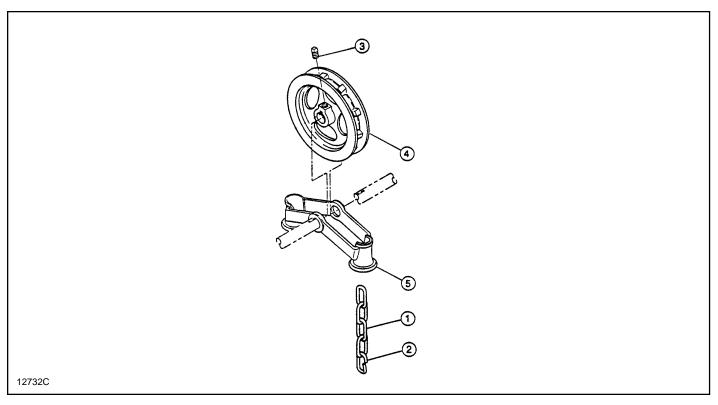
Figure 4. Hand Chain Drive. (Catalog Numbers 8282, 913115 and 332189-3)
