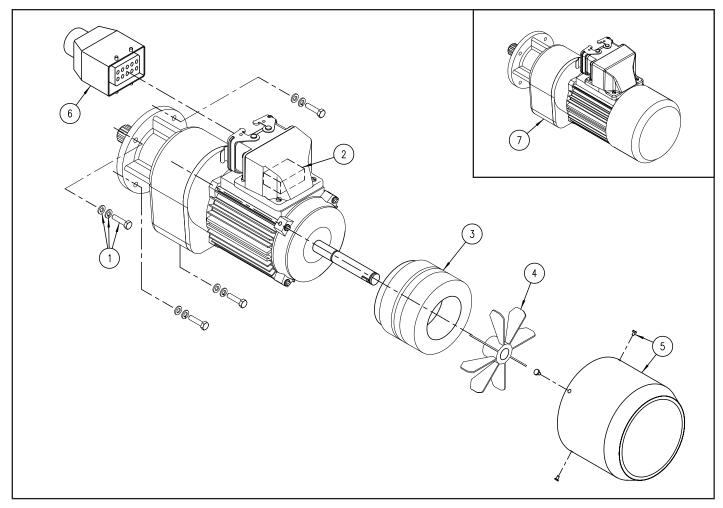
Figure 8. Gearmotor
