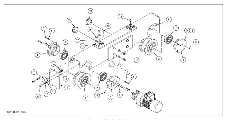
Figure 7. End Truck Assembly
