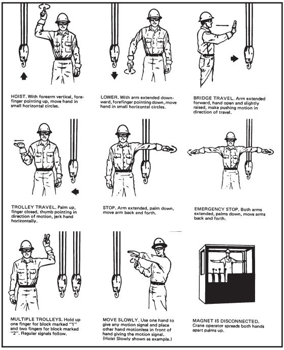
Figure 2. Operator Hand Signals
