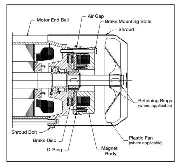
Figure 6. Motor Brake
