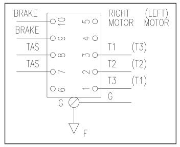
Figure 1. Bridge Gear Motor Quick Connection Plug
