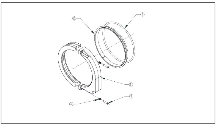
Figure 9-7. Rope Guide Assembly
