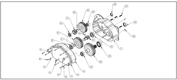
Figure 9-2. Hoist Gearing
