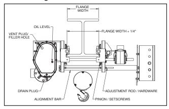
Figure 2-1. Trolley Wheel Spacing
