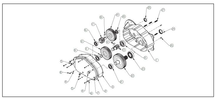
Figure 9-2. Hoist Gearing
