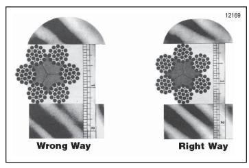
Figure 5-4. Correct Method of Measuring Rope
