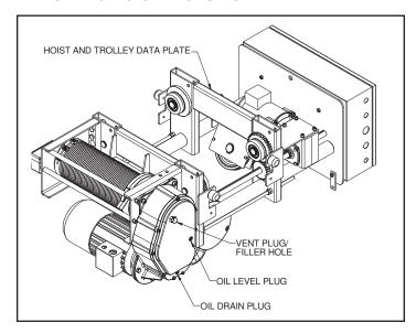
Figure 4-1. View of Hoist Showing Location of Name Plates and Oil Plugs
