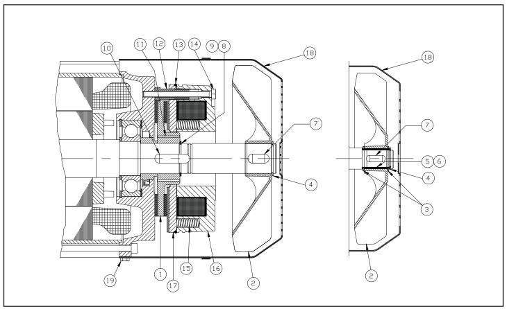
Figure 9-8. Standard Hoist Motor Brake
