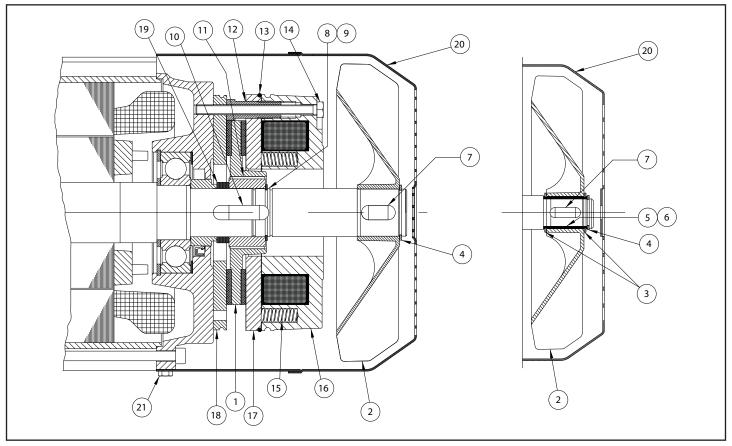
Figure 9-9. Outdoor Service Hoist Motor Brake
