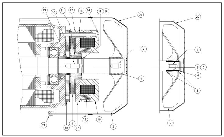
Figure 9-9. Outdoor Service Hoist Motor Brake
