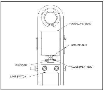
Figure 7-3. Over-Capacity Limit Switch
