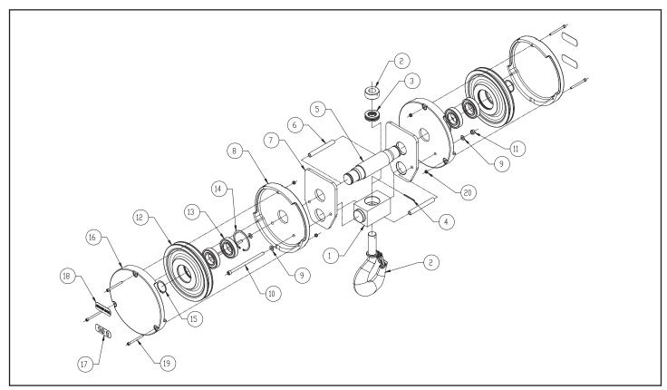
Figure 9-4a. Lower Block Assembly
