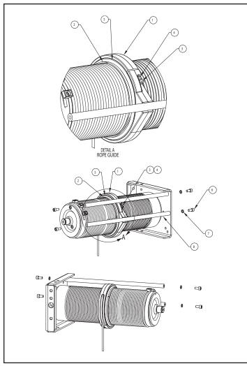
Figure 5-3 Rope Guide Assembly
