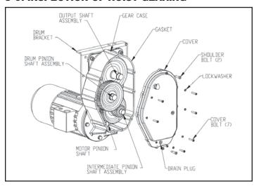
Figure 5-7. Hoist Gear Case Assembly
