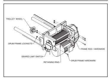
Figure 5-6. Drum Frame & Geared Limit Switch
