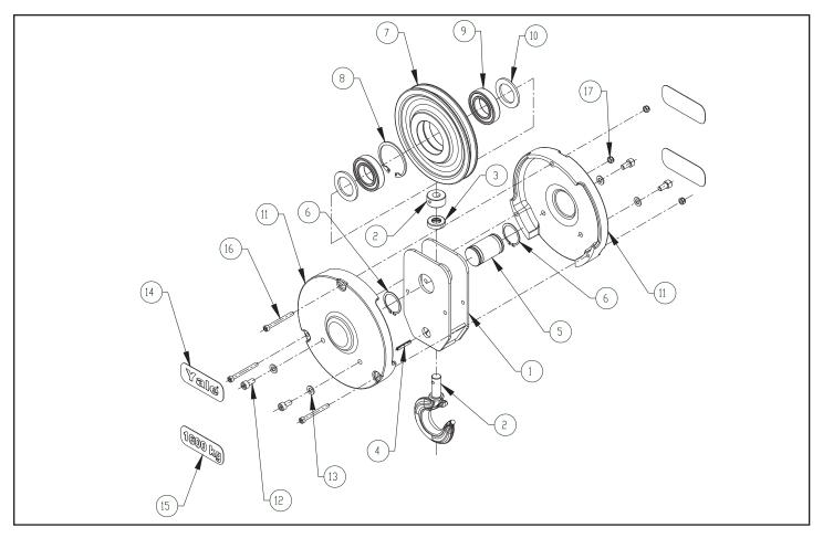
Figure 9-4b. Lower Block Assembly (S2 Reeved)
