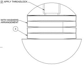
DETAIL A SPRING STACK (IN SERIES) DETAIL SCALE: (4 : 1)
