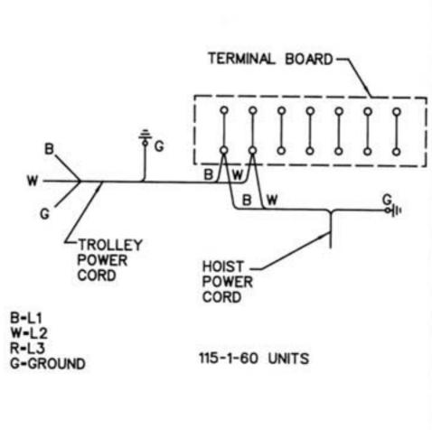
FIGURE 3. HOIST POWER CORD CONNECTIONS
