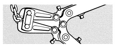
FIGURE 23. Cutting Chain with a Bolt Cutter
