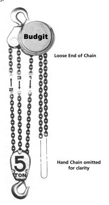
FIGURE 19. Reeving 5-6 Ton Hoists
