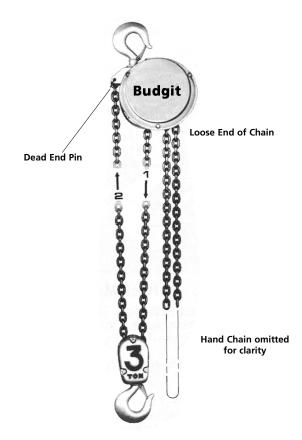
FIGURE 18. Reeving 3-4 Ton Hoists
