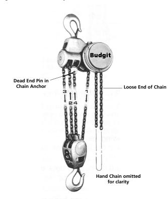
FIGURE 20. Reeving 8 Ton Hoists
