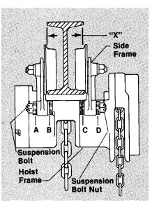
FIGURE 5. Trolley Spacer Arrangement
