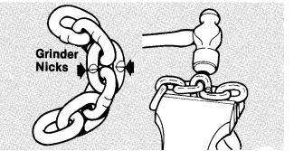
FIGURE 22. Cutting Chain by Nicking
