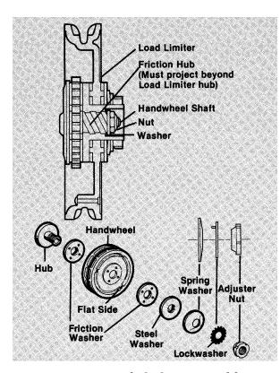
FIGURE 11. Load Limiter Assembly
