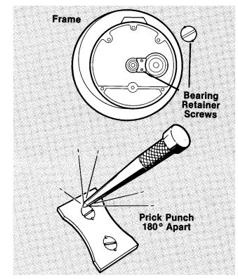
FIGURE 13. Bearing Retainer Screw
