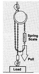
FIGURE 12. Load Limiter Calibration
