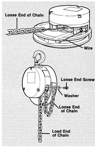
FIGURE 16. Reeving 1/4-1/2-1 Ton Hoists
