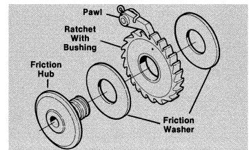
FIGURE 10. Brake Assembly
