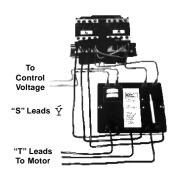
These two photographs are shown to provide a pictorial representation of proper wiring. Note placement of wires 40A and 41A to electrical interlock side of contactors with characteristic "X" of wires between electrical interlocks and contactor coil.
