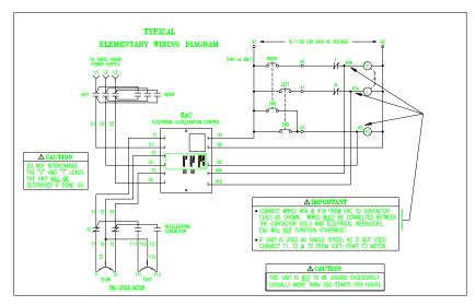
This Wiring Diagram is located on the bottom side of the Nema 1 enclosure cover. The steps listed above and notes located on the label must be followed for correct EAC installation.
