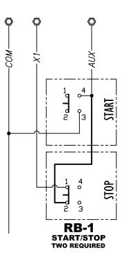
PUSH-BUTTON INSERT RATING: 125 VAC, ONE AMP CONTINUOUS PER CONTACT
