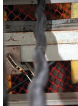
Failing cable due to the “corkscrew” effect
