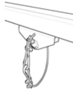
Diagram 11C. Safety cable installed on Gorbel® trolley that will attach to hoist (by others).
